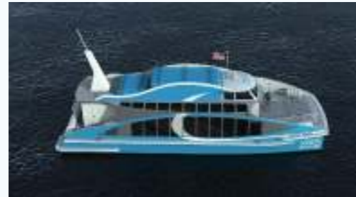
Golden Gate Zero 360kW FC, Operation 2019
